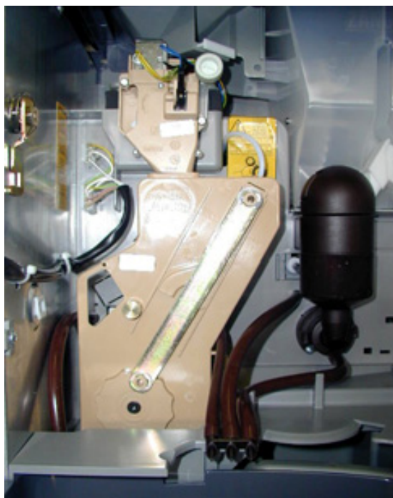
Espresso coffee brewer detail Positioned at the upper dead centre Ready for loading ground coffee
